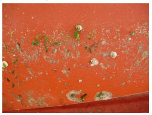
One problem the team observed when the boat ing. was pulled out was that the paint appeared to be damaged around one side of the water line. For more information on the boat or the paint, This may have been a result of the boat hitting contact Katy Wolf at IRTA at (323) 656-1121. or bumping up against the dock. The team agreed that the boat should be pulled out at a
